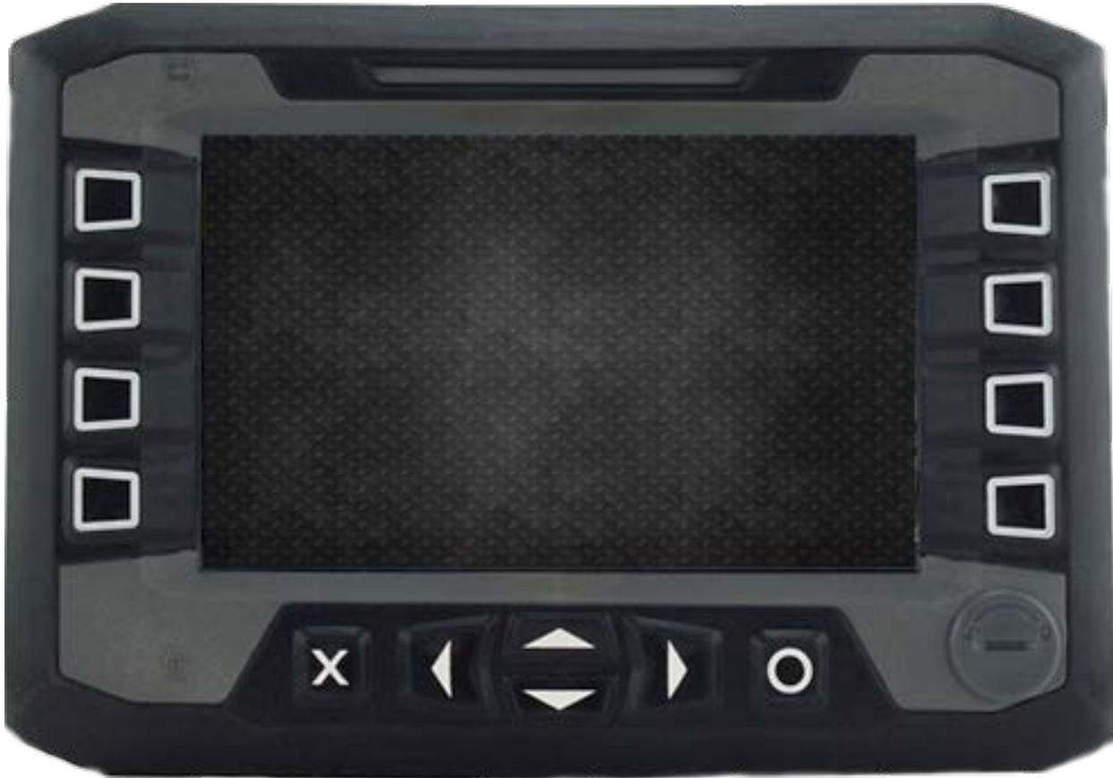
The Danfoss DP720 Monitor (DP720) is the communications interface between the operator and the CAN Bus system used to control the machine operation. From Key On until Key Off, the DP720 is a constant source of information.
