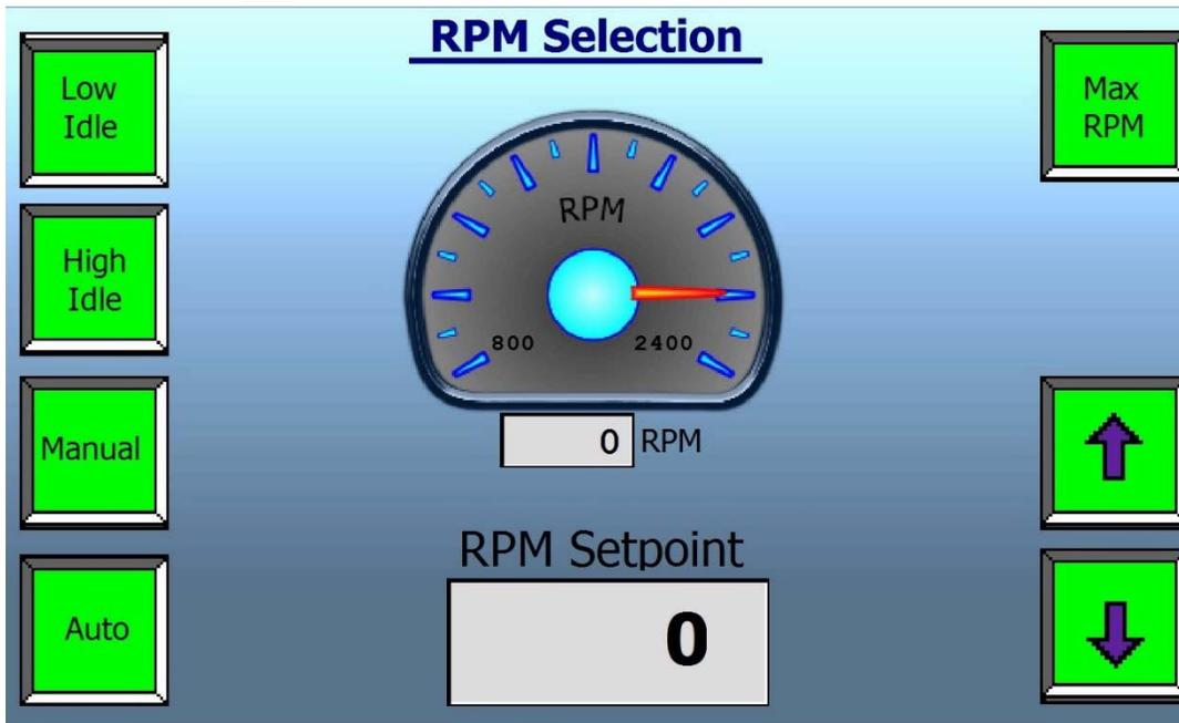
Low Idle: Sets Engine speed to 1200 RPM.
