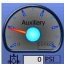
Auxiliary Gauge: The pressure required to Steer, Auger, Lift, Swing, AC, etc. All functions besides propel. 300-400 PSI on this gauge is normal when at idle.
