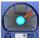
Charge Gauge: Displays the Charge Pressure of the Propel Pump. Approximately 350 PSI is normal. The pressure should maintain during forward or reverse propel.
