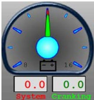
The T-644 has two batteries. Each is represented by a separate indicator on the dial.
