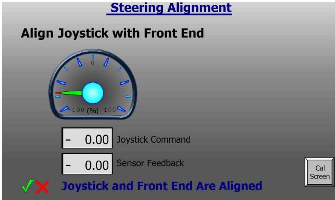
The Steering Alignment screen compares the Joystick steer command to the Front End position.
