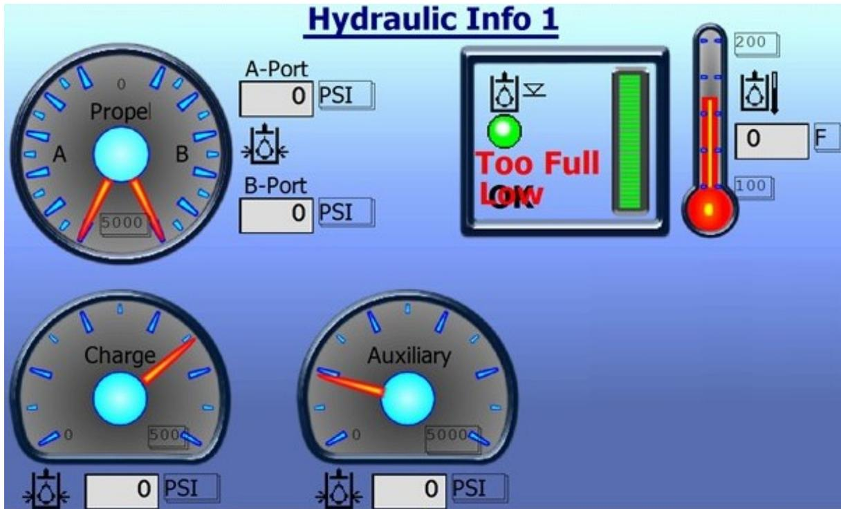
The T-644 has two main hydraulic pumps. Mounted directly to the engine is the Propel Pump, followed by the Auxiliary Pump. The Auxiliary Pump handles all other functions besides Propel.
