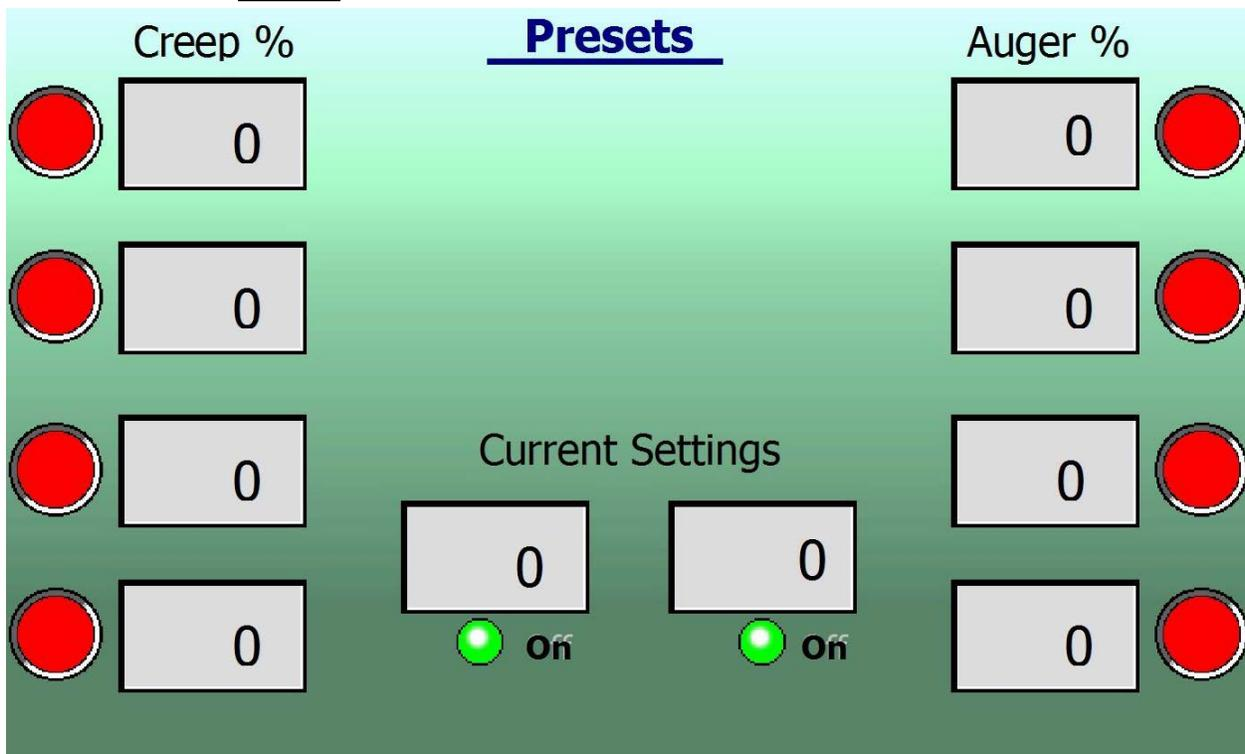
The Presets screen functions like the radio memory buttons in your vehicle. Save up to 4 Creep and 4 Auger settings for fast adjustment.
