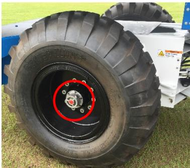
Gear Lube level should be between lines.
