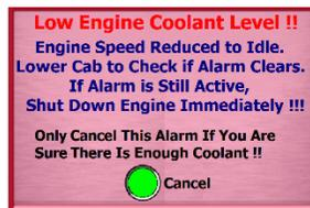
Low Engine Coolant Level: A loose or blown radiator hose or heater hose can be the cause. Only override this alarm if you have checked for leaky equipment.
