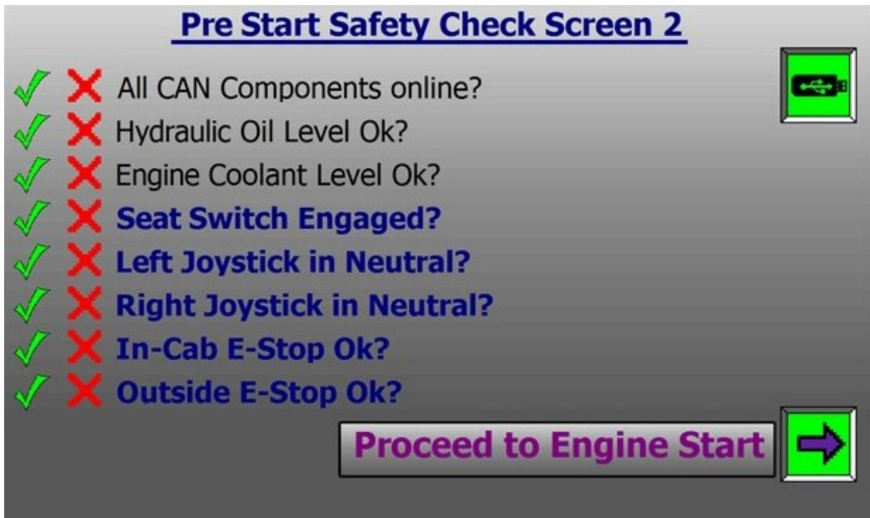
The Pre Start Safety Check Screen 2 displays the status of critical components prior to the machine start.
