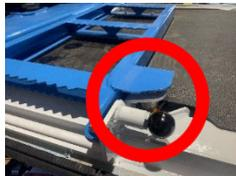
The Engine Bay Service Platform Ladder Sensor will not allow the Engine Bay Back Door to close IF the Ladder is unfolded. The Engine Bay Hydraulic Power Unit will run, but the cylinder will not move.
