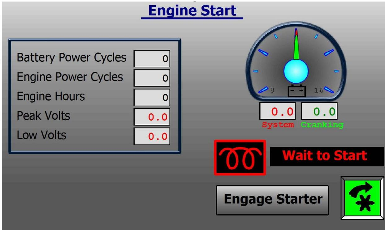
The Engine Start screen is where the Starter button is located.
