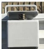
The Chute Cover Door Sensors will stop Auger rotation if a door is opened. The Chute Cover Doors must remain closed for the Auger to turn. Keep the sensor surface clean and avoid impact for maximum sensor life. A 3/8" gap is standard between the door and sensor.
