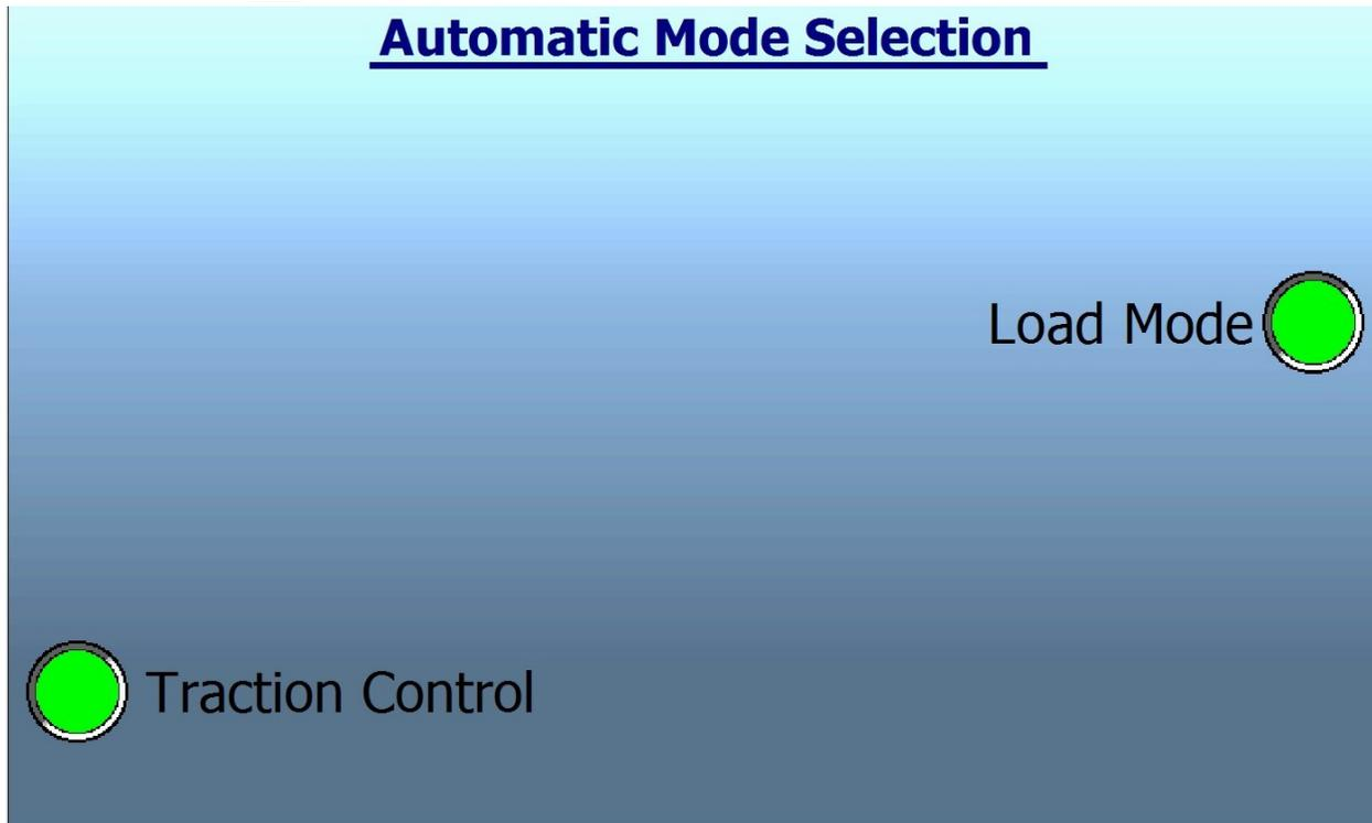
Traction Control: A software solution to help avoid tire slip. Green circle when enabled, Gray when off. It remains enabled, even after Key cycles, until turned off.
