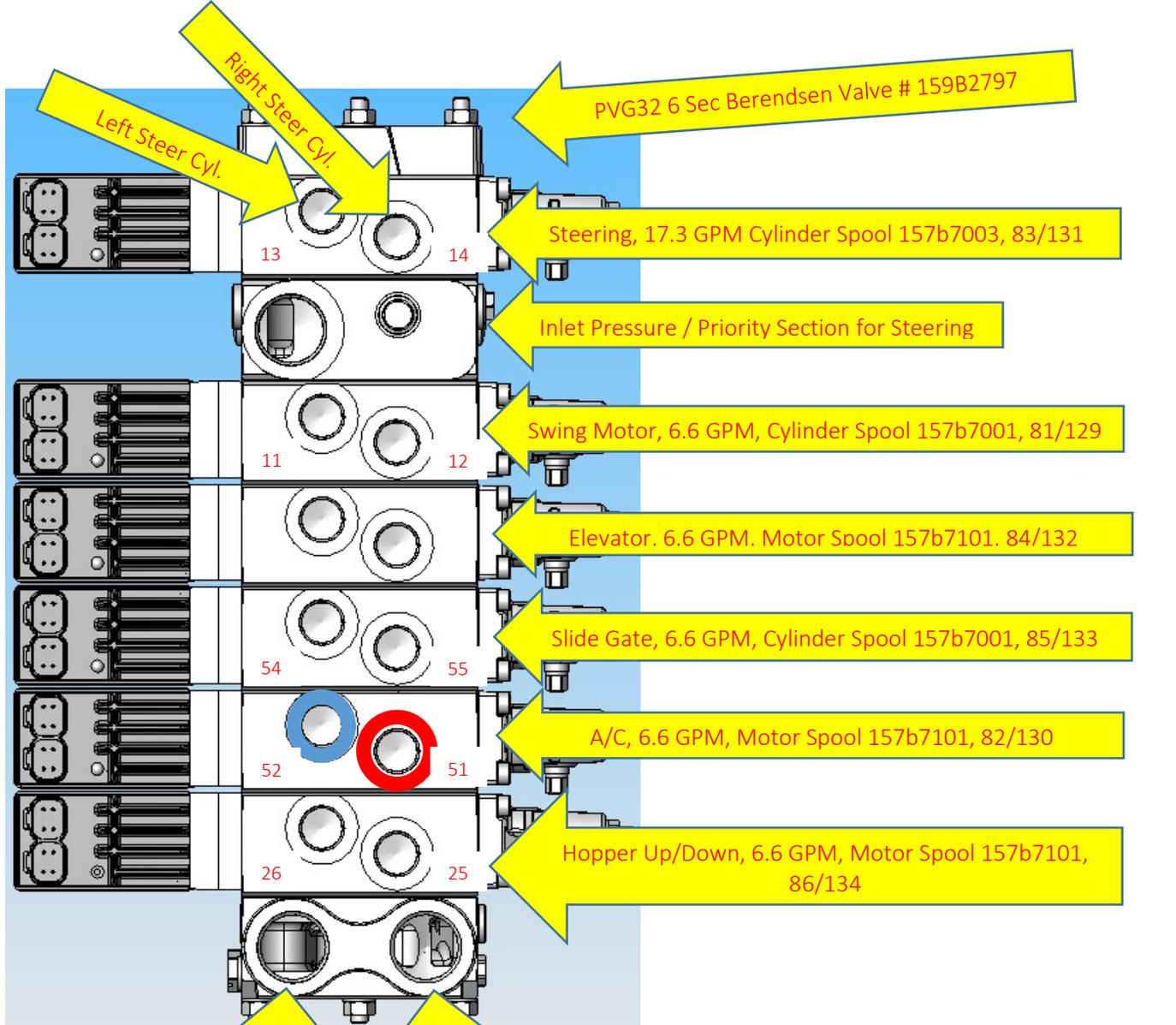
Valves Hydraulic oil supplied by, Danfoss Ser. 45, 130cc Pump
